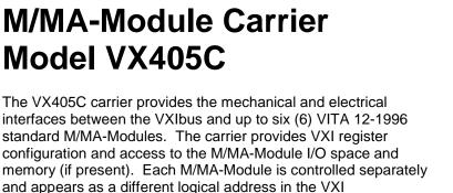
environment. Over 100 M/MA-Modules are available that can provide custom interfacing to the unit under test (UUT). Up to six
